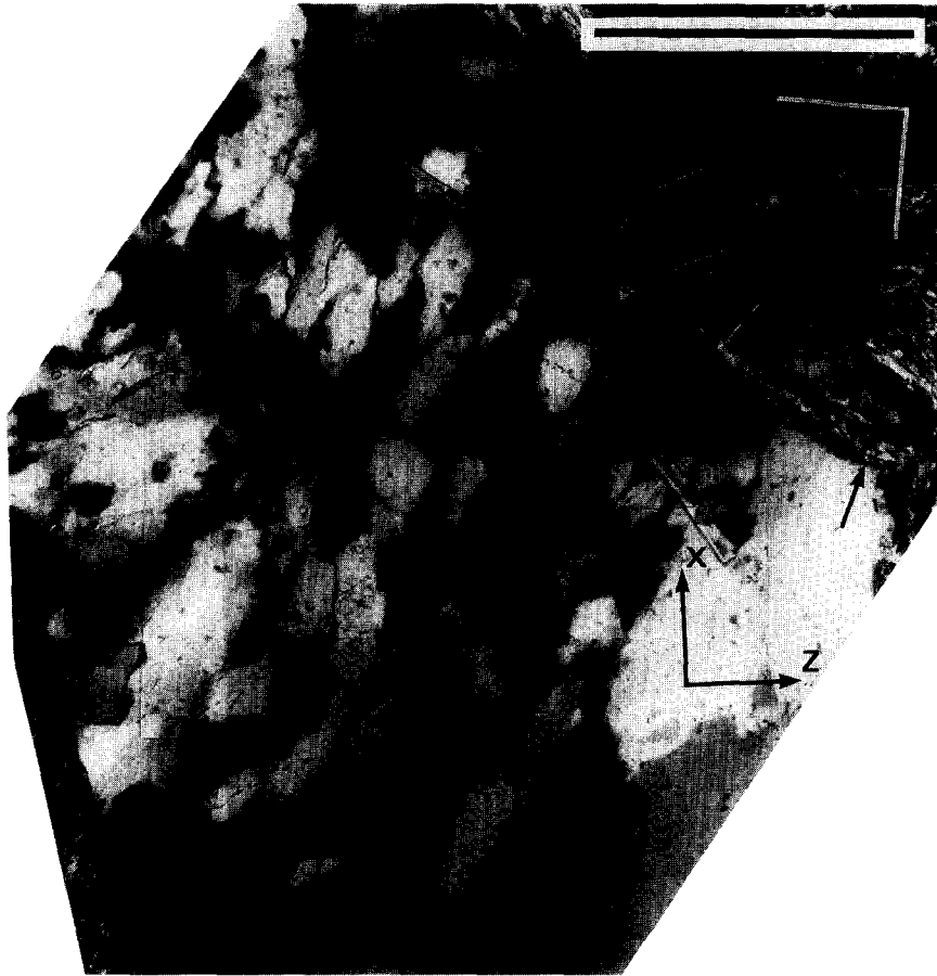
Fig. 9. Grain shape fabric in a part of domain 1.C of the buckled quartz vein (micrograph). Location is indicated in the inset diagram of Fig. 2. Note the shape preferred orientation of recrystallized grains, and the embayed vein matrix interface shown by arrows and a left-over grain (L) which were presumably caused by dissolution of the quartz vein (see text). Vibration directions of crossed nicols are indicated by thick bars. Scale bar = 0.2 mm.
